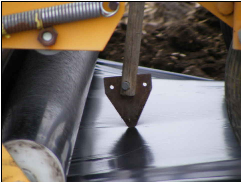
Detail of the tool used to cut slits in the plastic mulch
